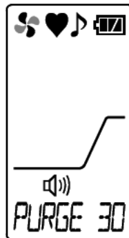
Automatic exhaust start (PURGE 30)
